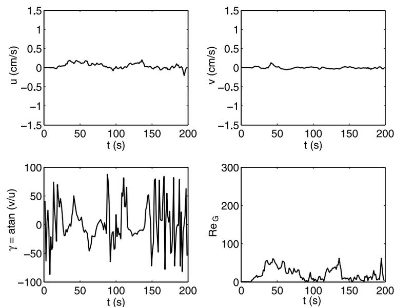
**Figure 11.** Time series of the velocity components,  $u$  and  $v$ , the direction of the velocity vector,  $\gamma$ , and the Reynolds number for an experiment with  $G/d = 0.29$  and  $y/g = 2.6$  in which dipole formation was not observed.
