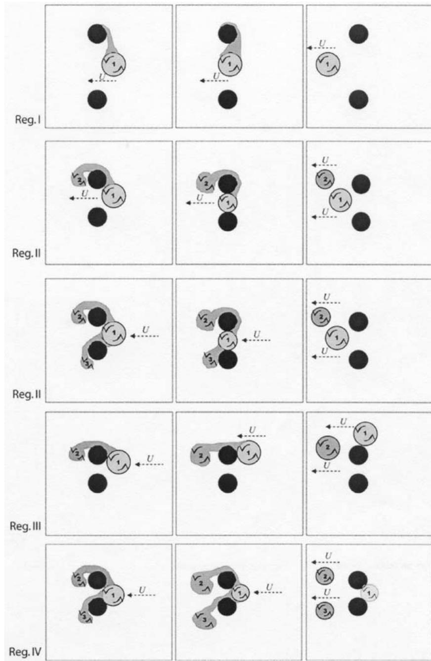
**Figure 4.** Sketch illustrating a self-propagating cyclonic vortex interacting with two cylinders for four different regimes discussed in section 3. The vortex self-propagated westward at a velocity  $U$  indicated by the dashed arrow. The original vortex is indicated by a 1, and the new vortices are indicated by 2 and 3.
