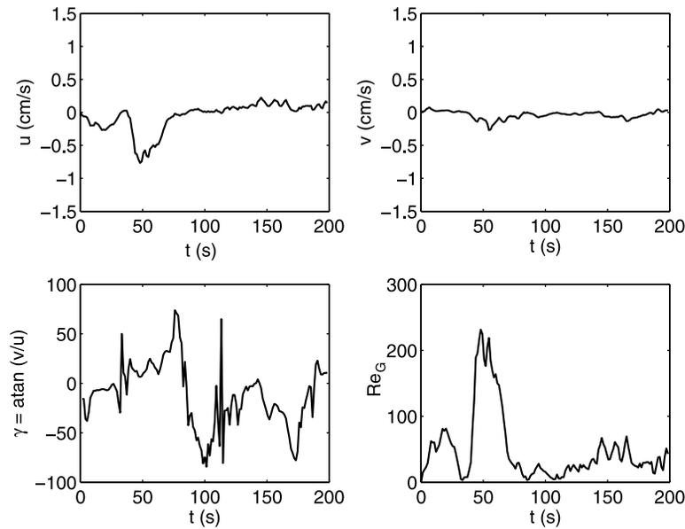
**Figure 10.** Time series of the velocity components,  $u$  and  $v$ , the direction of the velocity vector,  $\gamma$ , and the Reynolds number for an experiment with  $G/d = 0.3$  and  $y/g = -0.43$  in which dipole formation was observed.
