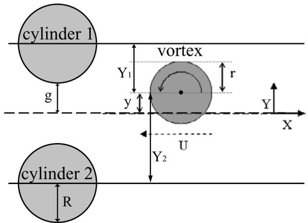
**Figure 3.** Sketch illustrating the geometry of the encounter between the vortex and two cylinders. The ratio  $y/g$  is a measure of the geometry of the interaction. For  $y/g > 0$  ( $y/g < 0$ ) the interaction takes place in the northern (southern) side of the gap, and for  $y/g = 0$ , the interaction is central.
