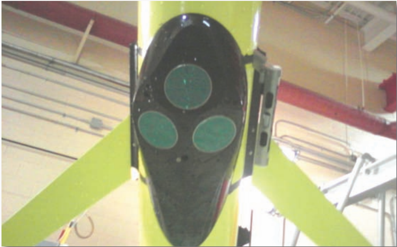
Figure 3 View of 400 kHz Nortek Aquadopp Profiler mounted on the underside of a Webb Slocum glider operated by researchers at Memorial University.
